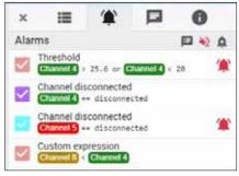
run a specified application such as an email or SMS client, and automatically annotate the capture graph to mark when the alarm happened and its duration. Alarms can also trigger a digital output on devices with supporting hardware, such as the PicoLog 1000 Series, ADC-24 and DrDAQ. You can even trigger a digital output from one of these devices based on an alarm condition from another connected logger without digital outputs, such as a TC-08.
