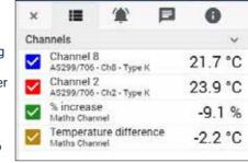
equation builder to perform simple calculations such as A-B, or more complex functions such as log, sqrt, abs, round, min, max, mean and median. Math channels are treated like any normal channel, so you can perform functions like alarms, graphing and annotations on them.
